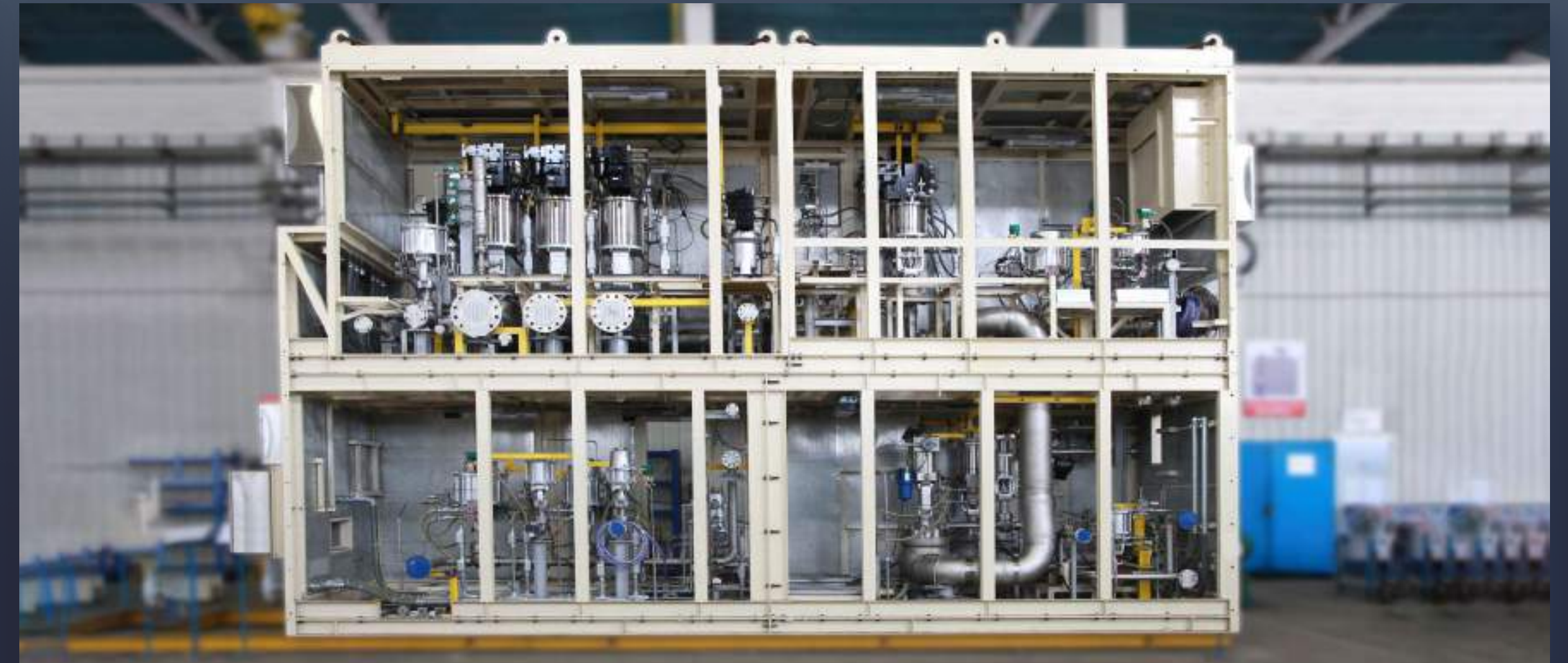
MITSUBISHI POWER 501J FUEL GAS & PURGE AIR ASSEMBLIES
